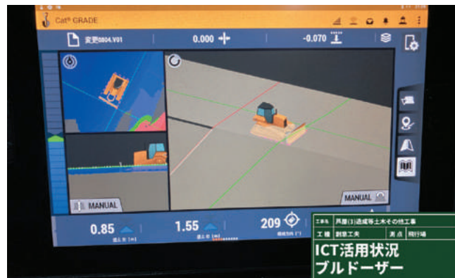
3D machine guidance screen on ICT-equipped bulldozer
