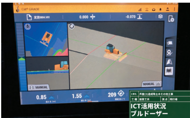
3D machine guidance screen on ICT-equipped bulldozer
