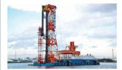
A Cement Deep Mixing method. This method hardens soft foundations by mixing soft soil with a stabilization agent in-situ using a rotating mixing shaft with blades. The method is suitable for providing stable strength quickly in both onshore and offshore works and for various purposes such as massive constructions, narrow space construction and treatment of contaminated soil.
