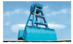
A large-scale wide bucket used for effectively carrying out highly precise shallow layer dredging. This equipment is tightly sealed and has a high soil concentration ratio per grab and the trajectory of the bucket blades can be verified on a screen from the control room while carrying out highly precise shallow layer dredging.
