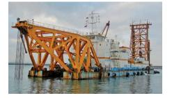
A dredging vessel which excavates sea bottom foundations using the cutter on the tip of the rudder, and dredges large quantities using its pumps. Dredged material is directly transported to the designated discharge areas through soil exhaust pipes. Our company has carried out continual improvement of dredging machinery since the company's founding in order to allow handling of dredging in a wide variety of soil qualities from soft mud to hard soil.
