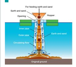
The Double Tremie Method is used for dumping sand into the sea. Because circulation flow from the inner tube to the outer tube is induced by dumping sand, the occurrence of turbidity is reduced more than it is with an ordinary single tremie method.
