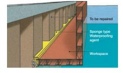
A technology for creating workspaces around waterside structures. A sponge type water proofing material is installed in the joints between the main structures and work structures which are then connected to create an air filled space in water. The technology provides superior waterproofing and strength properties and can handle even structures with very complex shapes allowing for repair and reinforcement construction to be carried out earlier.
