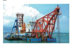
A dredging vessel which excavates sea bottom foundations using the cutter on the tip of the rudder, and dredges large quantities using its pumps. Dredged material is directly transported to the designated discharge areas through soil exhaust pipes. Our company has carried out continual improvement of dredging machinery since the company's founding in order to allow handling of dredging in a wide variety of soil qualities from soft mud to hard soil.
