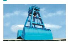
A large-scale wide bucket used for effectively carrying out highly precise shallow layer dredging. This equipment is tightly sealed and has a high soil concentration ratio per grab and the trajectory of the bucket blades can be verified on a screen from the control room while carrying out highly precise shallow layer dredging.
