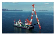
The company has constructed the "Kakuryu" large scale multiple angle swinging pile driving vessel with a 600t hoisting capacity and superior work efficiency to accommodate the increasing trend towards scaling up of diameter of steel pipe piles for the larger scaling of port facilities both in Japan and overseas.
