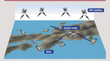
COS-NET (Construction On the Sea Network) is a system for monitoring and controlling work vessels through a combination of GPS and IT technology. Utilizing this system makes it easy to obtain accurate positions and other operation data.
