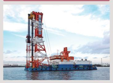
Koukaku is a special vessel designed for use with the CDM (Cement Deep Mixing) method, which is utilized to improve soft ground into a solid foundation suitable for the construction of a seawall, wharf, or quay. Koukaku is essential for providing stable support for large-scale structures. In addition, it is the first ecologically-oriented vessel equipped with a hybrid system that combines the high efficiency of fuel energy and natural energy.
