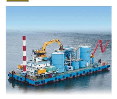
Production capacity: 360m³/hr of SGM light weight soil
