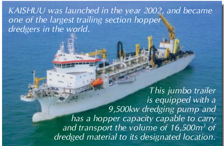
The two main engines of 8,000kw provides propulsion to a maximum speed of 16.5 knots.
